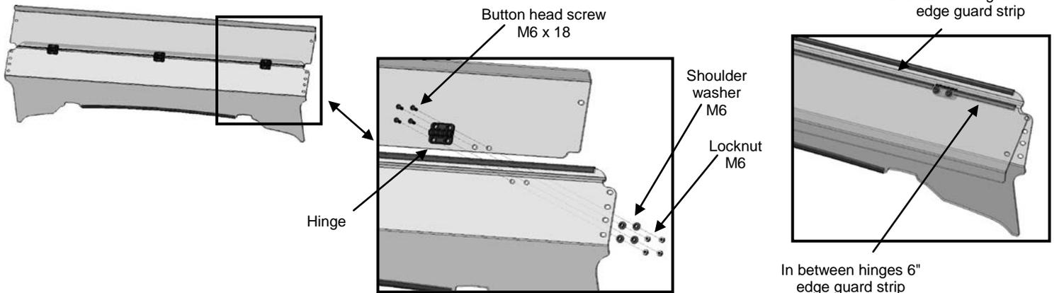
c) Attach clamps (Item E) & support arms (Item F) to the roll cage of your vehicle as per drawings. All clamps must be installed with the threaded inserts facing the front of the vehicle. **Do not tighten at this stage; you will need to make adjustments later on.**
