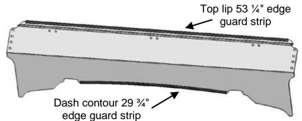
b) Assemble all hinges (Item D) to lower and upper windshield (Item A & B) as per drawings. **Optional: Install edge guard strip to upper shield in between hinges, this will eliminate any possible noise caused by vibrations.**
