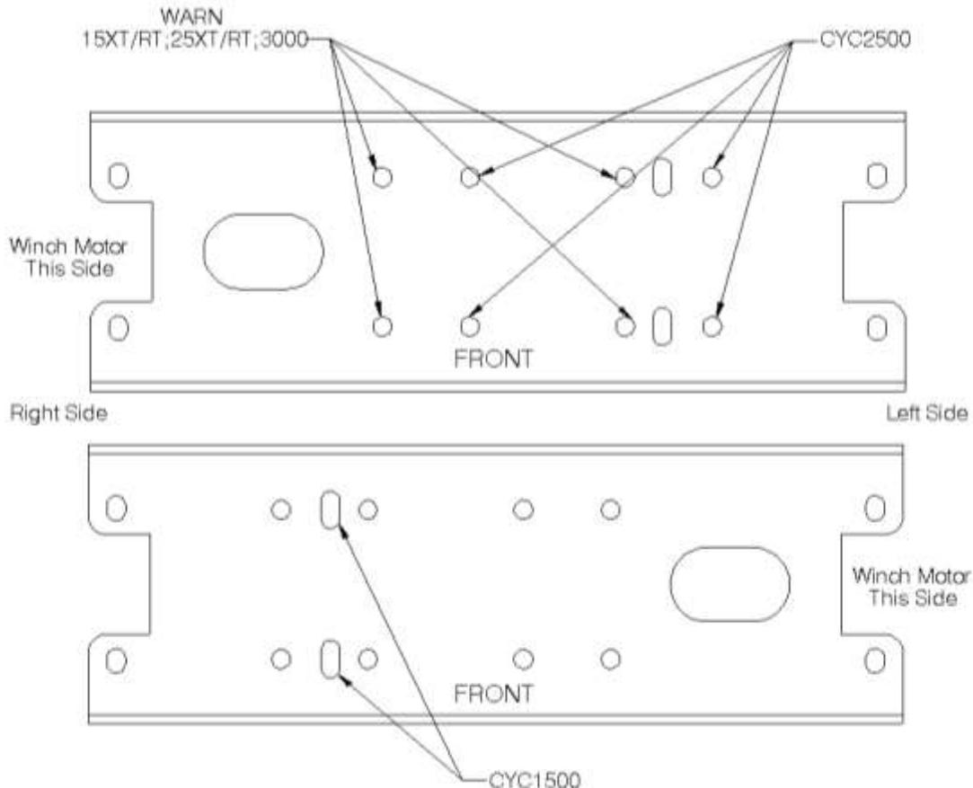
2. Install the two M8 x 25mm carriage bolts loosely into place on the winch adapter plate (Item 2) with flatwashers and nylock nuts as shown on the parts page. (These bolts need to be inserted into place now, because you may not be able to after the winch is installed.)
