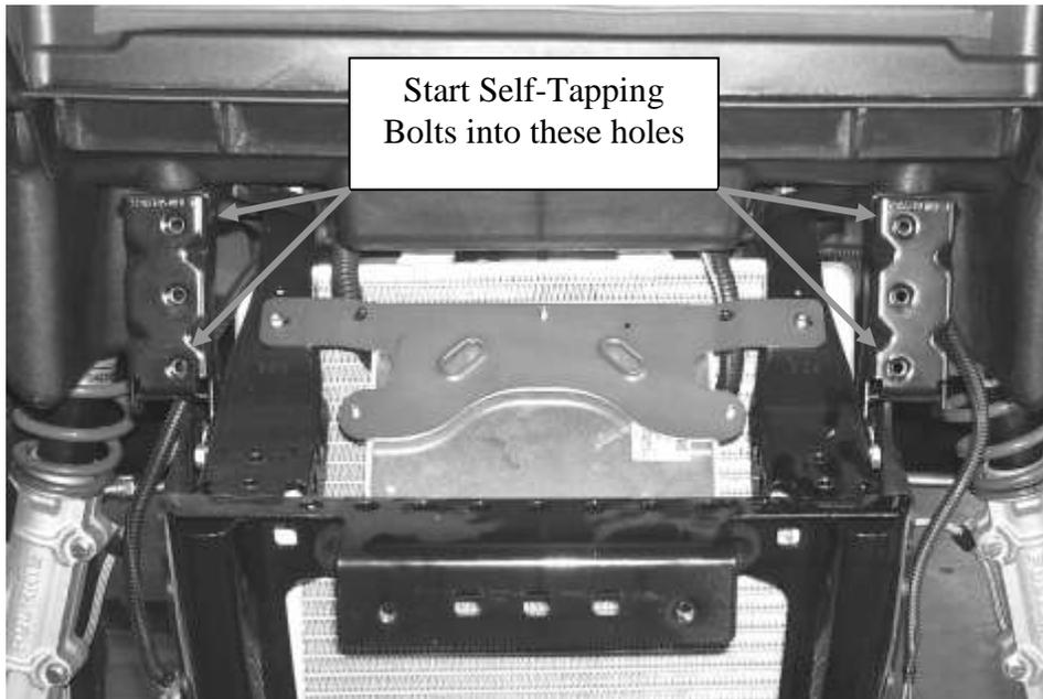
10. Route any wires through the wire access hole of the winch mount plate before installing winch assembly. Set the winch assembly into place on the ATV and install the four self-tapping bolts.
