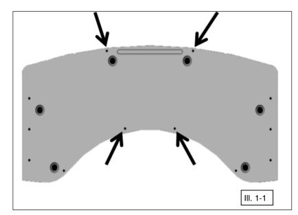
2. Attach mount plate to ATV rack using hardware provided in the mount kit. Do not tighten at this time. (See illustration 1-2).
